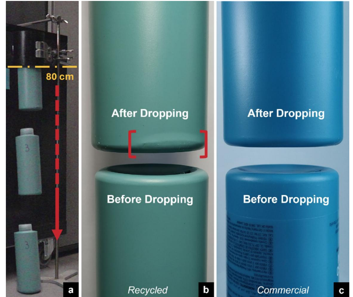
a) Drop test; b) Bulging on a recycled bottle; c) The base of a new bottle, showing no change
