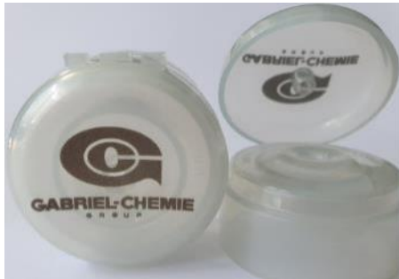
Laser marking on transparent polymers
